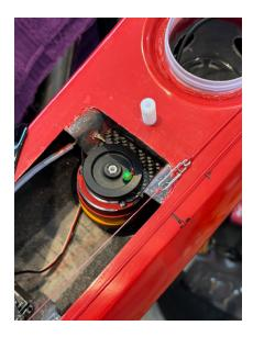
TIP: carefully remount the drum and cable up. My suggestion is don't put the securing screw back on the drum.... Just yet.
