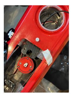
Now set the joystick fully out, secure the winch into the boat, make final checks of the winch turns, the cables the screws and re-mount the new winch to the bracket as shown above.
