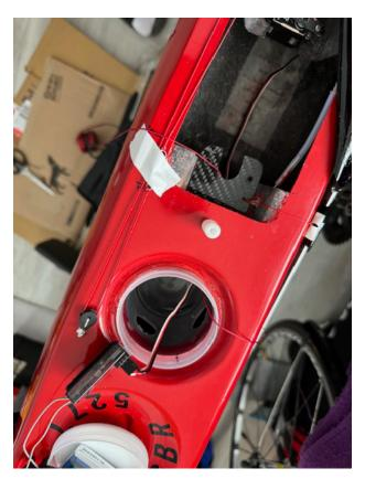
Unscrew the two retaining screws and lift the old winch out. Have a good look around to make sure the mainsheet and drum are still secure, plus the cable rethreading string/s are neatly available. Have a thorough inspection to make sure you understand everything down there before we load up again.
