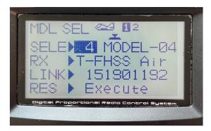
Need to begin a new boat/model? You can enter a new boat configuration, or take a copy of an existing boat and build upon that (see later in this manual). If you click on MDL SEL (Model select) with the JOG key, then keep clicking PLUS until you find an empty model slot. In this example, the first three slots already had boats in them, but number four is free. We would use this one as an example to add a new boat.
