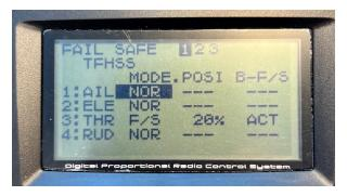
The factory standard for an airplane is to leave all the controls flying as set – which is probably straight ahead – except drop the plane's engine power to 20%. That's what you see here on the standard screen.
