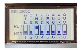
More Useful functions in the menu system include this REVERS screen above where you can change the polarity of your joysticks if you need. In this example, you can see that Channel 3 ("Mainsheet" in radio sailing) and here labelled THRottle, has had its polarity reversed to get the mainsheet direction of travel that we require.
