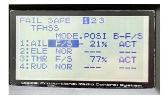
These are the proposed failsafe settings for sailing – helm part to port and mainsheet partly out. (see above photo)
