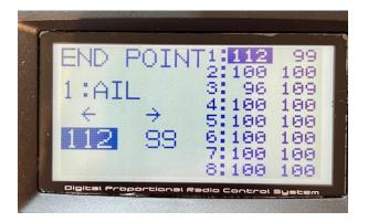
Adjust the values here on channel 3 to see the mainsheet take off hook on the boat adjusting itself to match your new numbers.
