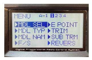
If you want to set up a new boat, the transmitter is preloaded with 30 model numbers. You can also see here (below) in this screen where you click to enter or alter a Model (Boat) name – MDL NAM
