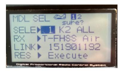
Can you see the word "sure?" on the screen above. The transmitter will now double check and invite you to confirm that this is the change you want, by clicking the JOG key again – a "beep" sounds to confirm the change is made. Press END a few times to revert to the main menu and double check that the correct boat name is on the screen.
