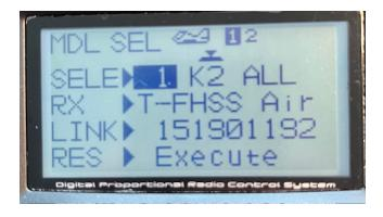
Can you see the black line with an inverted triangle on top? That is the transmitter saying that to select this model, you need to press the JOG key vertically down and hold
