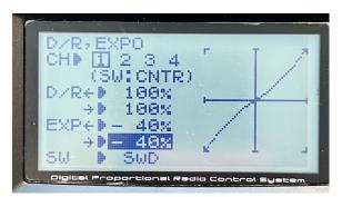
Note how the shape of the graph has moved from a straight line to an S shape.
