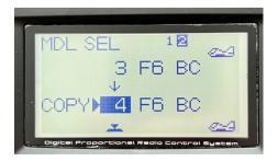
The new model you have created has all the same details as the boat you started with, including the name being the same. We want a new name for the new model. Now starting with the home screen set on your new model (Model 04 in my example), use the PLUS key for a second to get into the boat menus and select MDL NAM and use this
