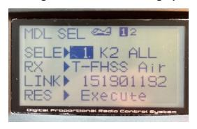
Can you see that the numeral 1 is highlighted in the large black box on the second menu row? . This indicates the transmitter is on model 1 – in this case the IOM named "K2 ALL"..
