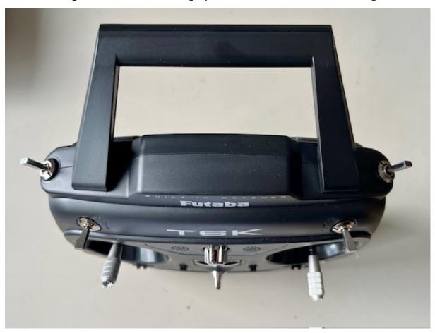
All four switches have three positions – up, middle, and down. This could become of interest if you want to experiment using one of the switches for "Rudder EXPO" or for "Pinch and Puff"
