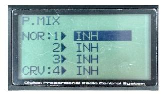
When you first look at the P.MIX screen it looks like this. You can Mix channels one to three, and put a Mix curve on Channel four. For Pinch and Puff mode we are ONLY going to adjust NOR:1 shown above. Get you cursor over it and click on the first field as shown.
