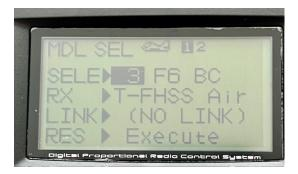
Nudge the JOG key to the left. You should get the COPY sub menu. You are going to copy the existing boat into the next free model slot available. Use the PLUS key to alter the model number in the copy location.
