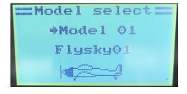
If you want to set up a new boat, the transmitter is preloaded with 20 model numbers. You can also see here (below) in this screen where you click to enter or alter a Model (Boat) name – MODEL NAME. You can change the name of a model quite easily using the selection of numbers and letters shown on the menu.
