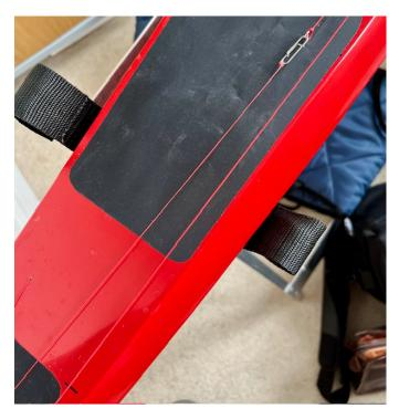
In this photo above the mainsheet is fully out and you can just see a tiny black mark in the top right corner of the photo near the steel hook, and the small black mark in the bottom left of the photo denoting the sheeted in position.
