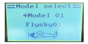
If you have a number of boats in the memory, you will be able to increment that line with the arrow (above) using the UP key, and skip through a selection of all the boats you have. When you have found the correct boat, click and hold the CANCEL key which effectively means "Save and Exit".
