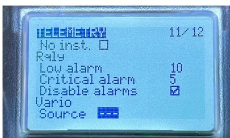
The Low and Critical alarm levels were originally assigned values of 45 and 42 respectively. I changed them (using the scroller) to 10 and 5 respectively. It seemed to make a small difference, but not much. So then I scrolled and clicked to put a tick in that box you can see labelled “Disable Alarms”. That appears to turn off this audible warning message pair completely.
