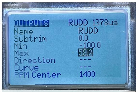
Using the scroller down to the number you wish to adjust and click. In this photo I have scrolled down to the maximum setting and clicked the scroller.
