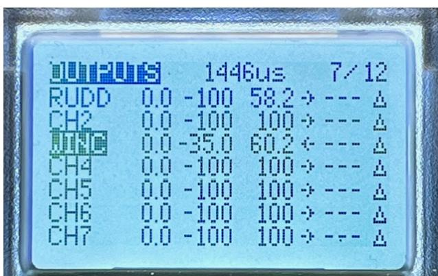
Now click on MDL, scroll to the boat you want in the list then click page forward to get to the OUTPUTS menu which is page 7 of 12. Scroll down to WINCH on channel 3 and click to select it. In this example you can see the limits are set at minus 35.0 and plus 60.2.
